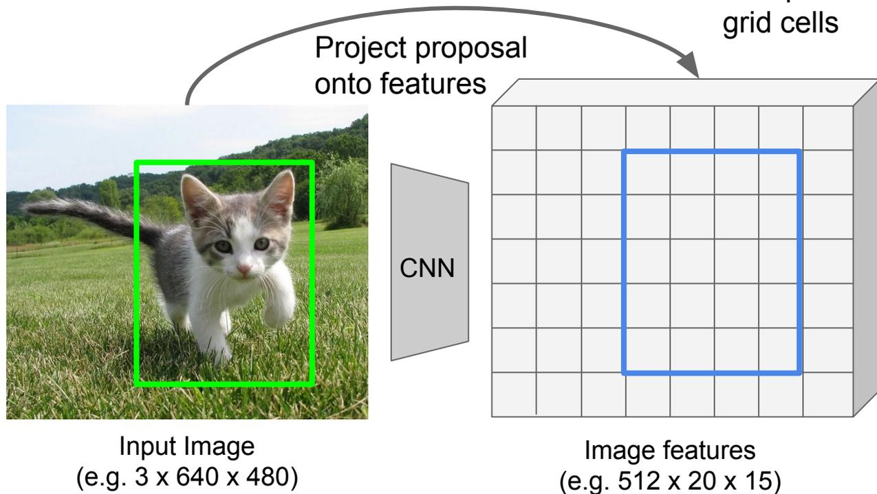
Q: how do we resize the 512 x 20 x 15 region to, e.g., a 512 x 2 x 2 tensor?
